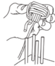
Fig. 10 Remove by unhooking stopper knot from notch & sliding loose monkey fist off of the posts.
